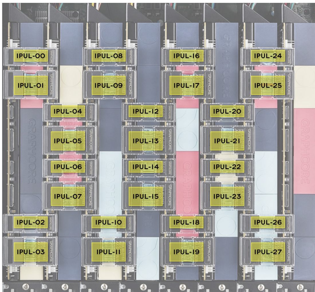
Fig. 17.2: IPU-Link card-to-card channel map
