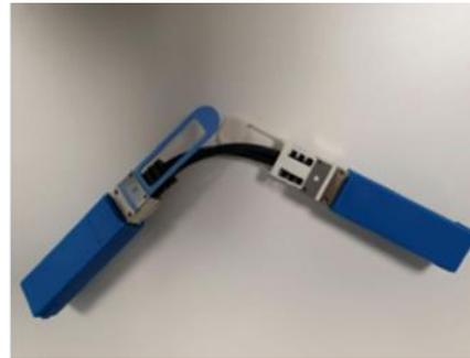
Before attempting to install the OSFP cables, it is beneficial to manipulate the cable to form a tight loop. During manufacture and shipping, the cables can form quite a stiff shape, so manipulating the cables before installing them reduces stresses on the socket during install.
