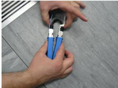
After installing a cable, pull gently on the black cable to ensure the plugs are firm in the sockets on the IPU-M2000.
