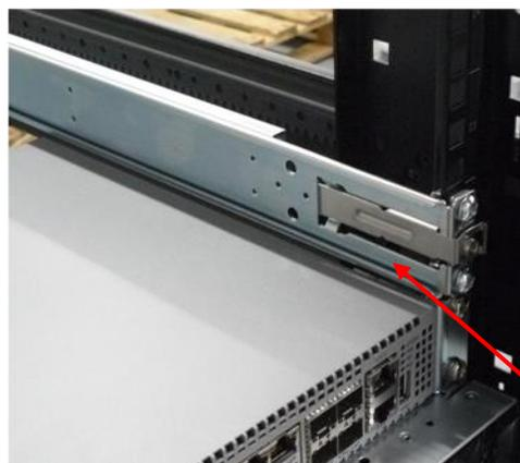
Insert the ToR switch ensuring the wheel on the switch is located in the groove on the slider.
