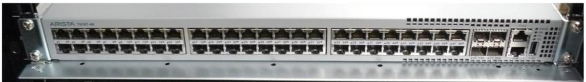
Place the management switch on top of the last IPU-M2000 and screw it into position using 4x M6 screws.
